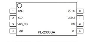
Figure 4-1 Pin Assignment Diagram of PL2303SA SOP8 Package
