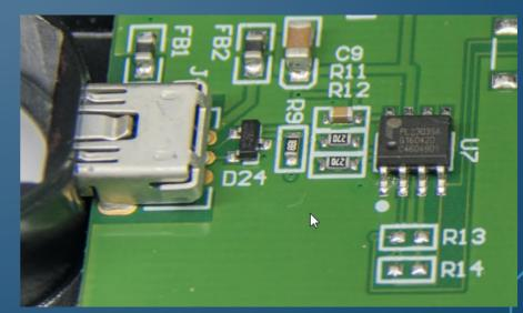
Soldering pads nearby → easy soldering
