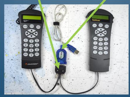
Serial Adapter to connect different Handcontrollers to a PC (not at the same time)
